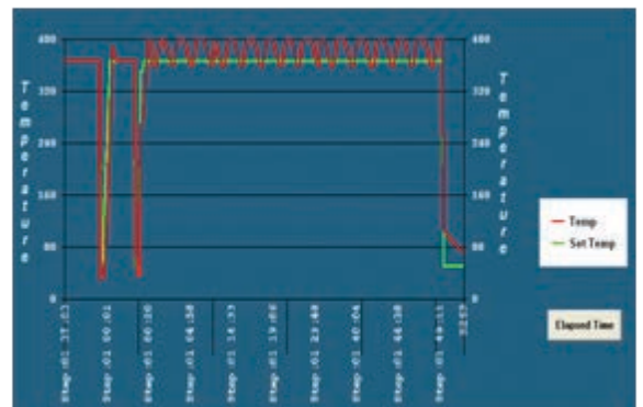
Programmed muffle furnace and temperature chart obtained
